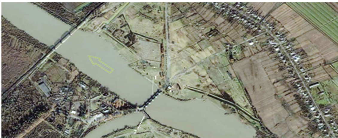
Fig.8. The water dividing dam on the river Rioni. 1– Dam; 2 – Gateway regulating the water supply from the river Rioni to the City Channel.
